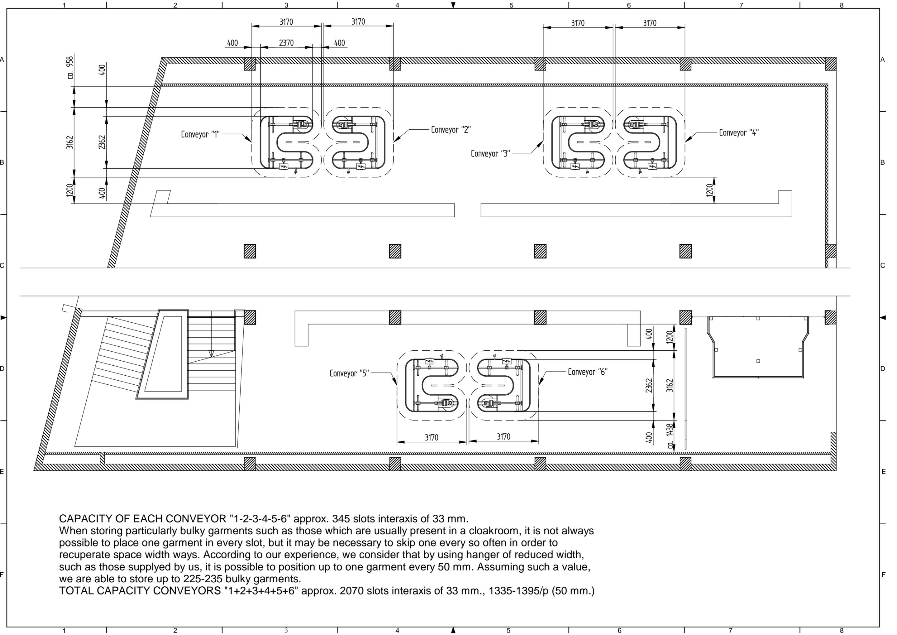
CAPACITY OF EACH CONVEYOR "1-2-3-4-5-6" approx. 345 slots interaxis of 33 mm.
